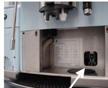
Main water tap
